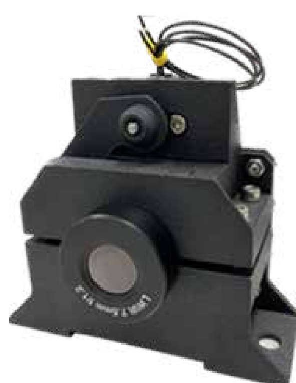
Figure 7. Photo of the ASTROtir breadboard. Within the 3D-printed housing, one can see the commercial lens in the front as well as a shutter mechanism slightly behind and above the lens.
