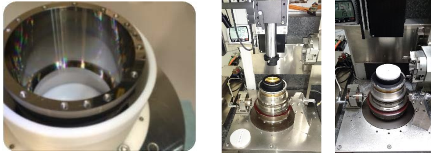
Figure 2-13: Left: Aluminum tubes plated with Ni and diamond turned –almost mirror quality
